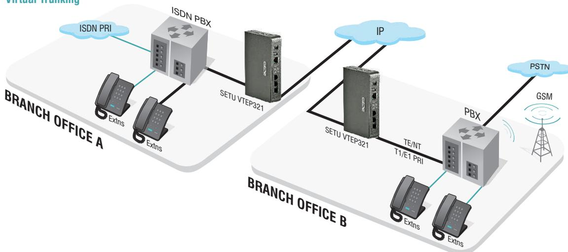
SETU VTEP enables users of one branch-office to virtually access trunk connectivity of the other branch office. SETU VTEP routes the call over cost-effective IP network till the last mile of termination and facilitates users at one location to access the local ISDN connectivity of remote branch-office to further reduce inter-network call charges.
