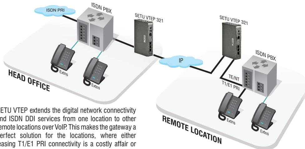
SETU VTEP extends the digital network connectivity and ISDN DDI services from one location to other remote locations over VoIP. This makes the gateway a perfect solution for the locations, where either leasing T1/E1 PRI connectivity is a costly affair or availability of fixed network is intricate.
