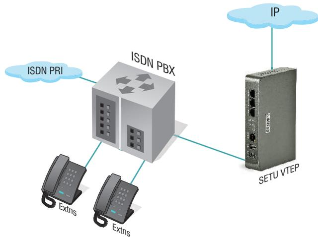
SETU VTEP transparently integrates with existing ISDN PBX using T1/E1 or PRI signaling to provide VoIP connectivity to existing PBX users. Programmable TE/NT modes ensure a hassle-free integration. Dedicated ports for network clock sync avoid synchronization errors and guarantee superior voice quality.
